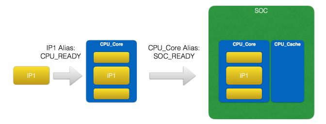
As shown, an IP (IP1) can be integrated by the CPU\_Core, which in turn can be integrated into the SoC - all of this is done using the moving aliases flow described above.
